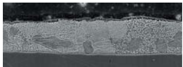
This micrograph of the Galvalloy coating shows the distribution of aluminium and zinc-rich phases.
