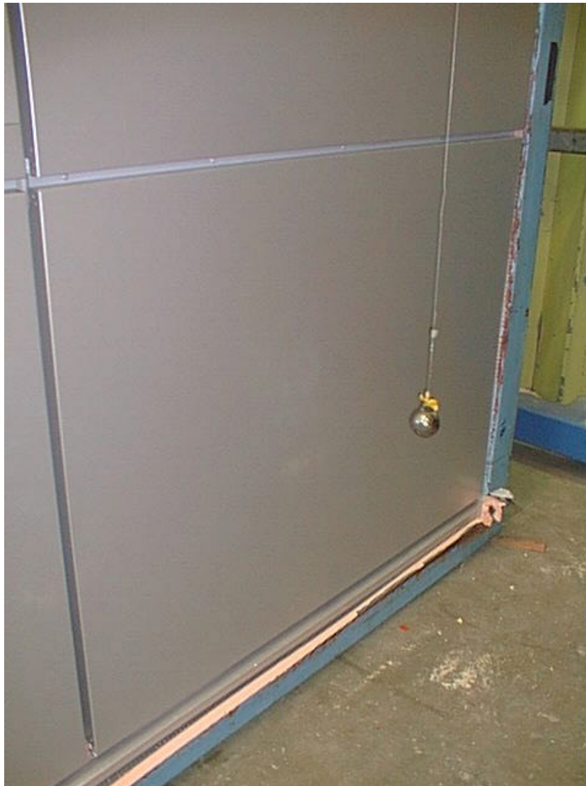
Figure A2. The indoor face of the test specimen wall showing a hard body impactor
